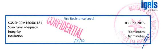
Testing undertaken by Intertek Shanghai testing facility to ASTM E119-16a where the equivalent standard fire curve was used in the boards evaluation.
