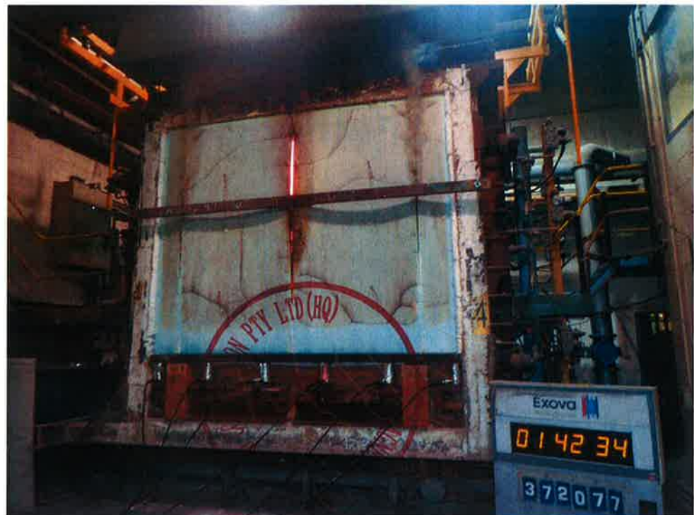
The unexposed face of the specimen after a test duration of 102 minutes
