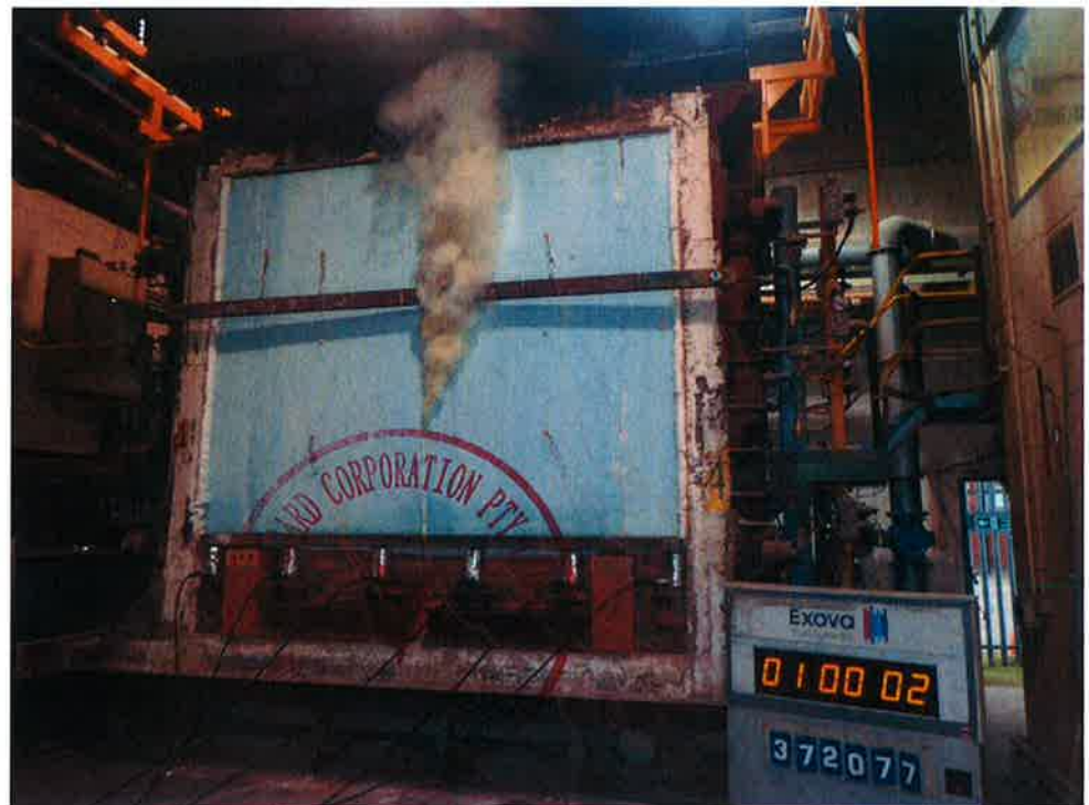
The unexposed face of the specimen after a test duration of 60 minutes
