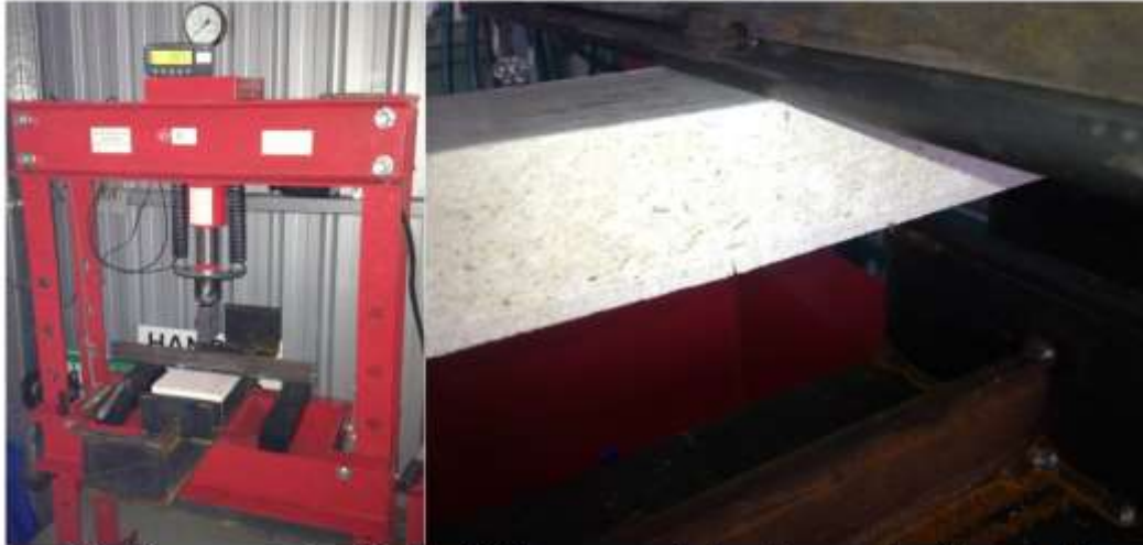
Testing apparatus. Typical failure: a crack develops under the sample
