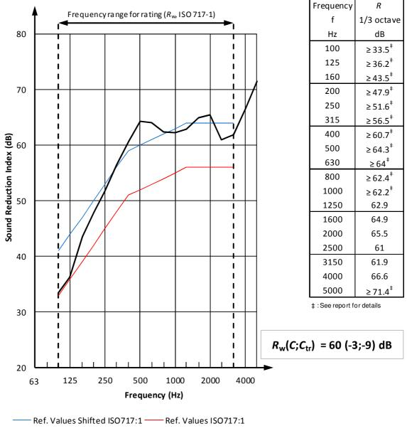
Evaluation based on laboratory measurement results obtained in one-third octave bands by an engineering method.
