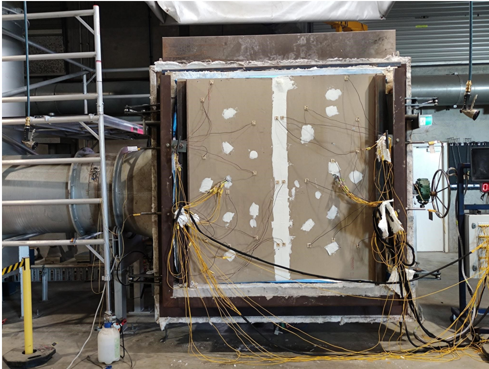
Photo 1 - Non-fire side before test
