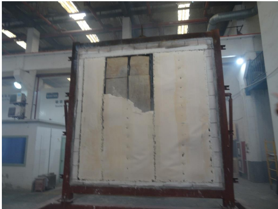
Photo No. 6 Exposed Side after 120 Minutes
