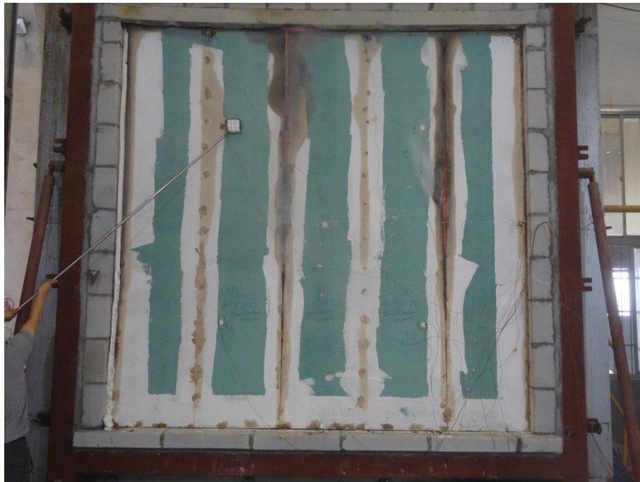
Photo No. 4 Unexposed Side after 102 Minutes
