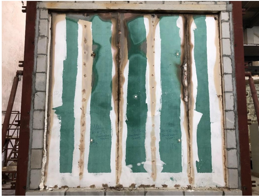
Photo No. 5 Unexposed Side after 120 Minutes
