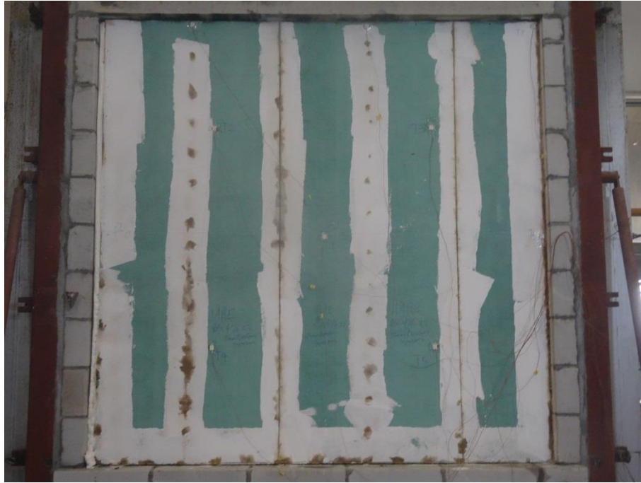
Photo No. 3 Unexposed Side after 31 Minutes
