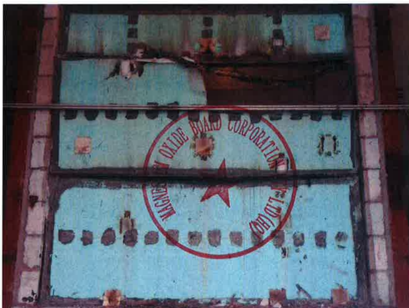
Fig. 14 - Unexposed Side after Hose Stream Test
