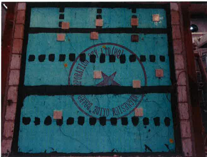
Fig. 2 - Unexposed Side Prior to the Fire Test
