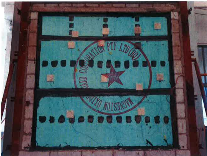
Fig. 4 - Unexposed Side after 60 Minutes
