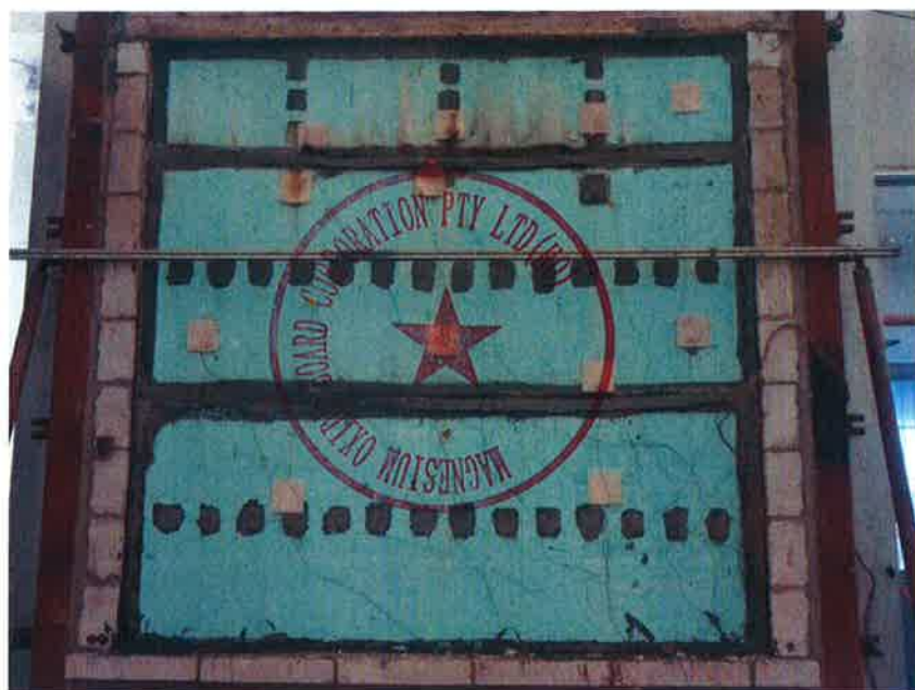
Fig. 6 - Unexposed Side after 150 Minutes
