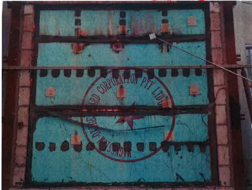
Fig. 7 - Unexposed Side after 180 Minutes
