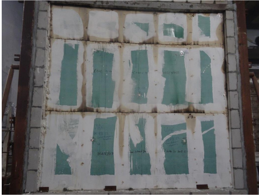
Photo No. 5 Unexposed Side after 120 Minutes
